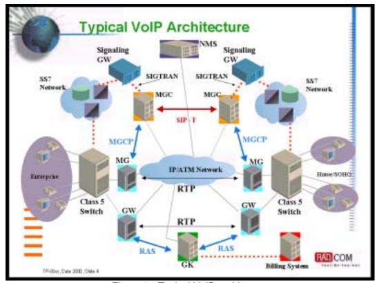
Figure 1 - Typical VoIP architecture
